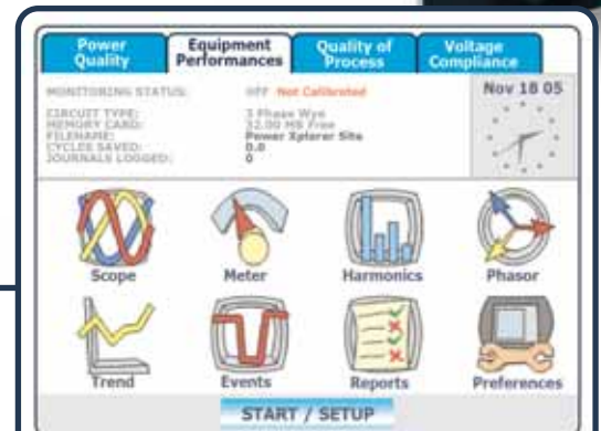
Optional local color touch display with tabs representing sample Encore applications
